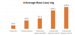
► TABER wear mass loss test (1000 cycles/1000g) TABER wear test follows the ASTM D4060 standard
