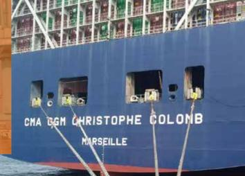
The rope is made of high-strength polyester and superpoly material with perfect proportion and twist. This product fully combines the advantages of the two materials and has a higher cost performance. Its high breaking strength and wear resistance are equivalent to 100% polyester fiber, but its weight is reduced by 20% concurrently, the rope is round and solid, with smooth surface and easy operation, which is a more efficient rope.
